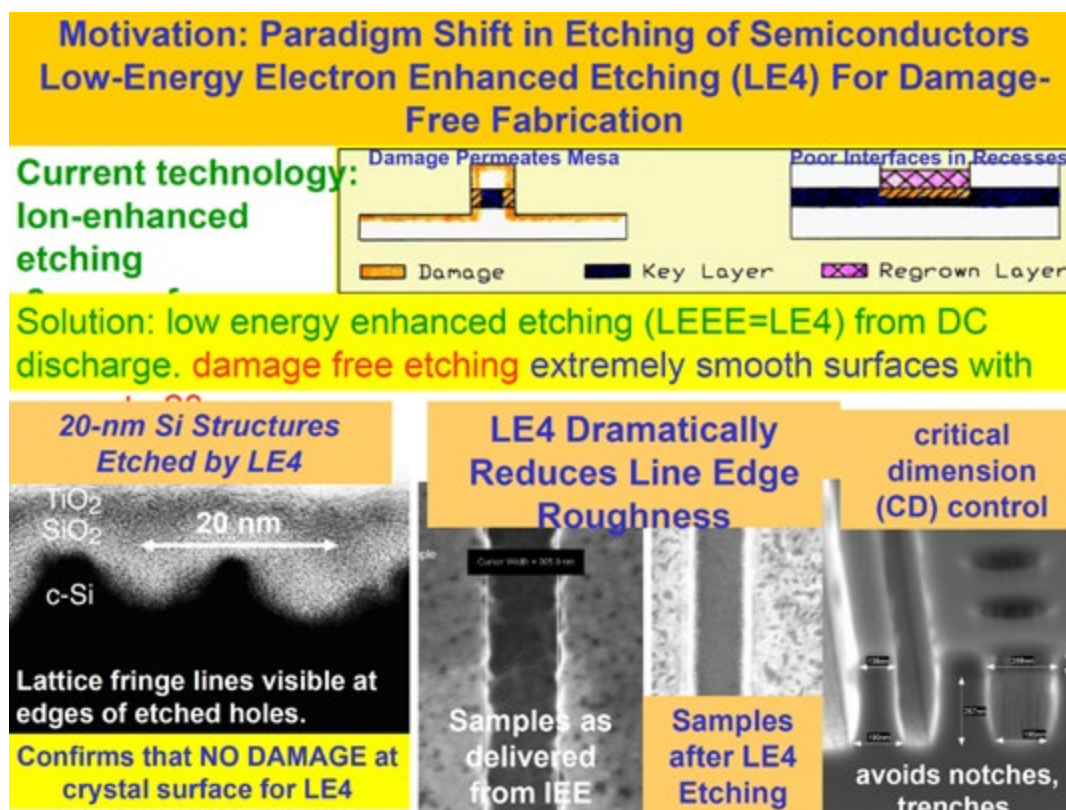
Figure 35. Damage-free fabrication of 20-nm silicon structures made using Low-Energy Electron Enhanced Etching (LE4) instead of Ion Enhanced Etching (IEE). Credit: William A. Goddard III, used with permission.
