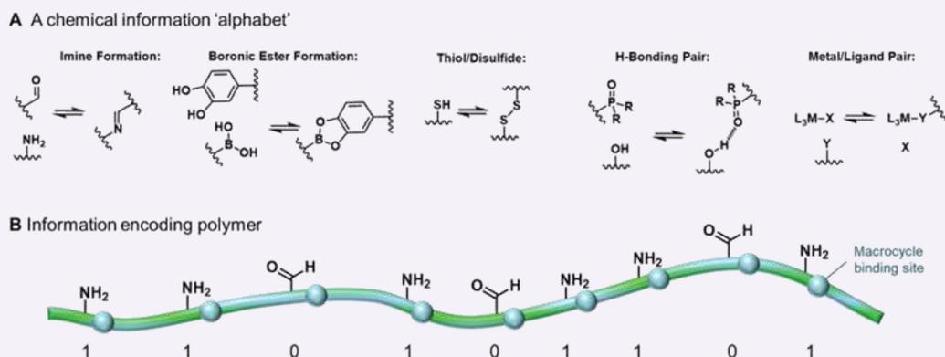
**Figure 1.** (A) A proposed compilation of several highly specific dynamic covalent interactions to be utilized in the 'alphabet' for information storage (Task 2). (B) use of two 'letters' from the 'alphabet' enables binary coding of information along an information-bearing polymer.
