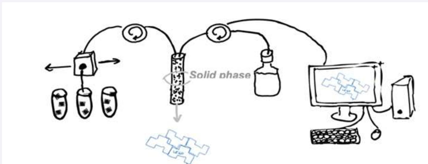
At each step of the construction, a solution containing the next building block is sent through the microfluidic channel for enough time that it is very likely one of those blocks has reached, and bound to, its matching position in the structure. Then the solution of remaining unbound blocks are flushed out and a solution with the next block is sent in.
