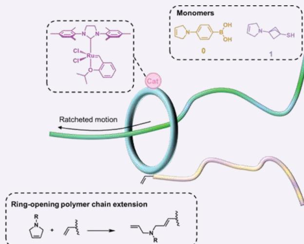
**Figure 2.** Task 3 and 4 might be performed by the same catalyst. Ring opening polymer chain extension via alkene metathesis is catalyzed by a Hoveyda-Grubbs Gen II catalyst. This extends the growing polymer and the energy release from this reaction can be harnessed to drive directional ratcheted motion of the information polymer.
